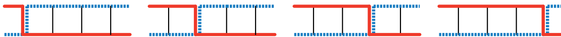
Fig. 2: The four pseudoline arrangements supported by the network \mathcal{X}_4 with two levels and four commutators.
